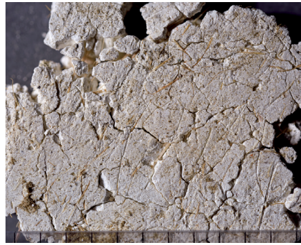
Fig. 12: Unpainted white lime plaster floor fragment from palace room E with characteristic fine plant fibres as organic fillers. Scale 2mm.
